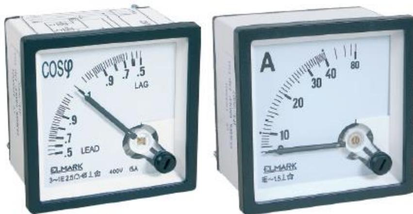
Analogue devices adjusted for mounting on the front panel of electrical boards. Designed for frequency measurement, capacity, alternating or direct voltage and current of the power supply grid, with overall dimensions 72x72mm. They are manufactured on the basis of bridge measurement schemes. There is possibility for display change for the higher scopes of measuring.
